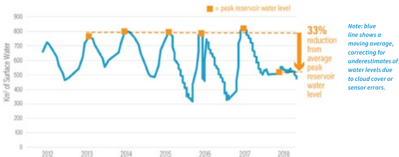
Figure 3-4 The area of Sagar Dam over time, showing water losses due to drought and water management changes (data from Deltares using monthly JRC water occurrence data for 1999-2015 and NASA/USGS, ESA satellite data for 2015-2018)
